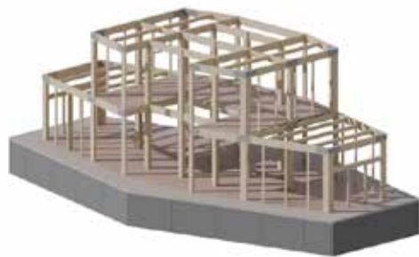
1) Structure Lightweight wooden structure on concrete ponton
